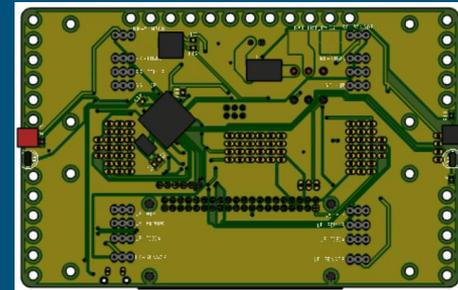
Figure 17: MicroDog PCB
