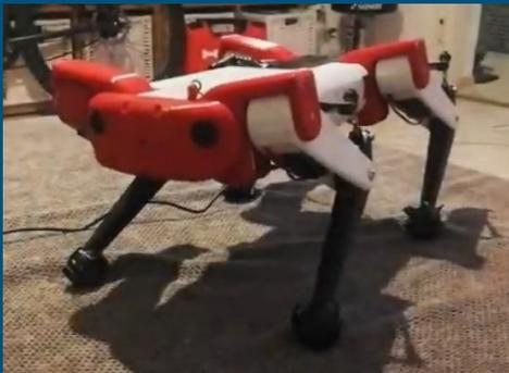
Figure 7: Robot with Force Feedback [7]
