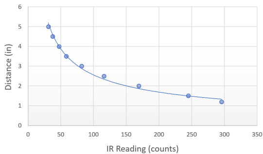
(b) Calibration curve translating the IR sensor readings into distance.
